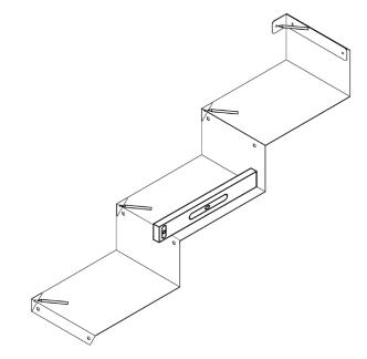
Drill the marks you made in step 4. Place anchors in holes.
